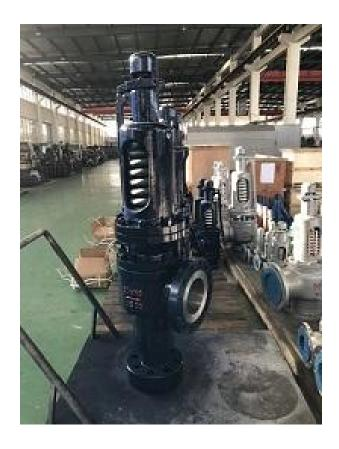
UAE Valve is known as the leading <u>Conventional Safety Valve supplier in UAE</u>. It is a kind of valve that releases excess pressure automatically to prevent damage or collapse to systems. It is a vital instrument that is used in a variety of industries to manage and reduce overpressure. Designed to protect pressurized equipment and devices, including boilers, pressure vessels, and pipelines, from overpressure situations.
